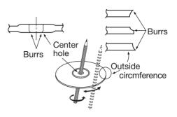
Remove all plastic particles of burr from surfaces of disc before loading in magazine.
